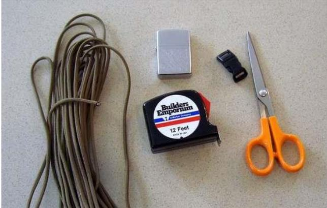
1. You'll need paracord, or equivalent 1/8" diameter cord, a tape measure or ruler, scissors, 5/8 side release buckle, and a lighter (torch lighter works best). The amount of cord used can vary, but for this example, we'll use 10 feet of paracord to start with. Actual amount of cord used for the bracelet is about 1 foot of cord for every 1 inch of knotted bracelet length. So if your wrist is 8 inches, you'd use approximately 8 feet of cord.
